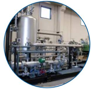
In modern PVC production plants liquid ring compressors work as strippers for the Vinyl Chloride gases, which are entirely recovered to be reintegrated in the production cycle. GARO VCM compressors are reliable and efficient machines, provided in both single and double stage versions according to process pressure requirements.
